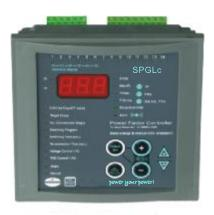
Reactive power compensation plants are used to decrease the load of cables and power distributions caused by inductive currents and to save reactive power costs. The power factor controller is a main part of such a plant and connects or disconnects capacitor stages automatically. The series SPGLc power factor controllers are suitable for the use in conventional or special dynamic reactive power compensation systems and a mixed operation is possible as well.
