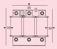
A spacing 30mm is necessary to ebsure proper cooling
