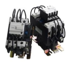
SPGL GMC contactor can be used in 400-690V, AC, 50-60Hz up to control 60Kvar capacitors, when a capacitance is switched to an AC system. The result is a resonant circuit damped to a greater or less degree. In addition to the nominal current, the capacitor accepts a transient current that is a multiple (as more than 200times) of its nominal current. Fast switching, low-bounce contactors should be used.
