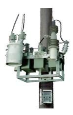
The series SPGLbTBB(p) Pole mouning Capacitor Banks are especially designed to compensate the reactive energy in power networks outdoor, like pole mounting for the normal load or with harmonics content. Permit the suitable using networks up to 24KV ungrounded (and 36KV grounded).
