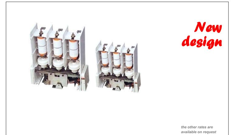
The air contactor uses a vacuum arc extinguishing chamber to extinguish the arc, which is used to frequently connect and cut off normal working current. It is usually used to remotely connect and disconnect 6KV, 10/12KV AC motors and capacitor bank with frequent starting and stopping of medium and low voltage.
