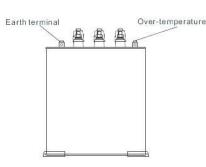
The main rates 230 to 1000V 50/60Hz up to 60Kvar 5Kvar,10Kvar,12.5Kvar,15Kvar,20Kvar,25Kvar, 30Kvar,40Kvar,50Kvar,60Kvar
